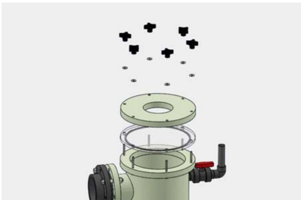
Figure 7-25: Flange at the filter casing
